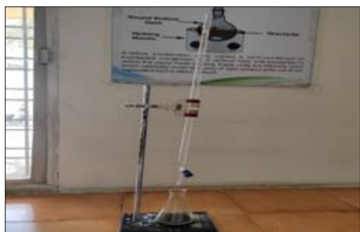
Figure No. 22:- Acid value determination
