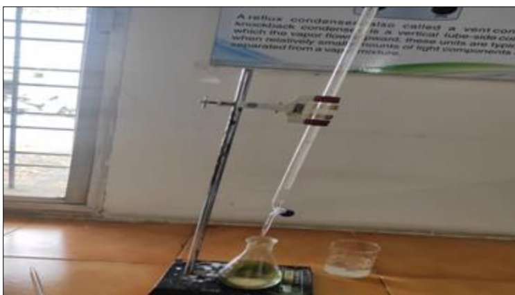
Figure No. 24:- Saponification value determination
